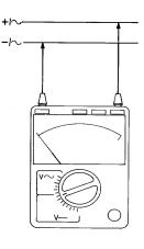
$\, \stackrel{\diamondsuit}{\circ} \,$  Read off the measured value: in the case of DC voltage, on the two upper scales 0 ... 5 or 0 ... 15 V, A ... , in that of AC voltage, on the scales beneath 0 ... 5 or 0 ... 15 V, A  $\sim$  .
